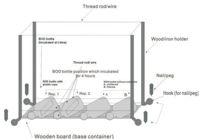
Fig 1 Design of incubation bottles in holder construction.
