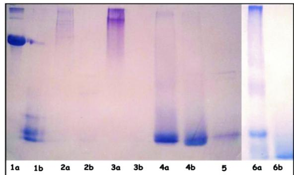
Fig 6 SDS/PAGE of hydrolysis products of proteases from *B. megaterium* DSM 319 on some proteins. 1a, BSA; 1b, hydrolyzed BSA; 2a, collagen; 2b, hydrolyzed collagen; 3a, gelatin; 3b, hydrolyzed gelatin; 4a, keratin; 4b, hydrolyzed keratin; 5, Protease protein (control); 6a, hemoglobin; 6b, hydrolyzed hemoglobin.
