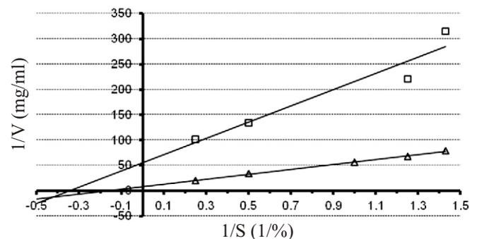
Fig 7 Kinetics of *B. megaterium* DSM319 proteases on gelatin ( $\Delta$ ) and albumin ( $\square$ ). The Lineweaver-Burk equation,  $r: 1/V=49.072(1/S)+8.0948$ ,  $R^2= 0.99$ ;  $\text{£}: 1/V=160.73(1/S)+55.235$ ,  $R^2=0.92$ .
