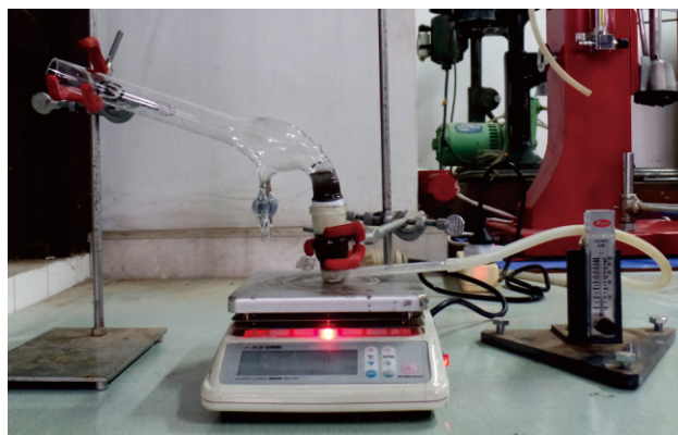
Fig 2 Photograph of a modified Hallimond Tube used for microflotation test.
