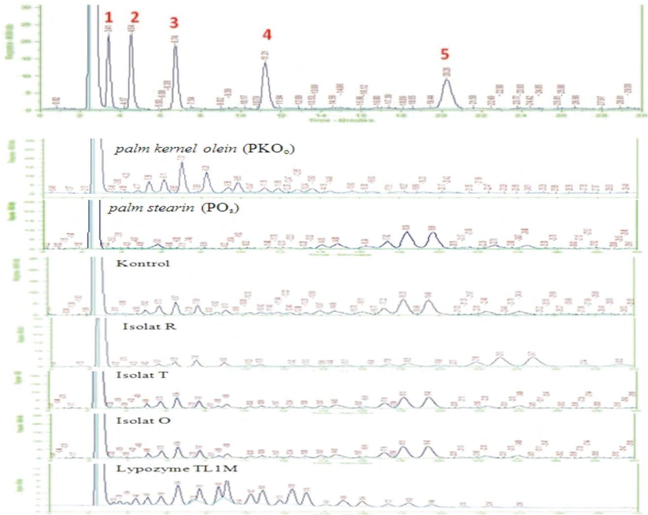
Fig 9 High Performance Liquid Chromatography (HPLC) analysis result. Triglyceride Mix Standart; Specification peak: [1]Glyceryl trioctanate; [2]Glyceryl tridecanoate; [3]Glyceryl tridodecanoate; [4] Glyceryl trimyrystate; [5]Glycerol tripalmitate.
